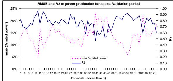
Figure 17:  $R^2$  and rmse of the power production forecasts for every forecast horizon and for the validation period.
