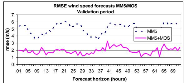
Figure 8. Rmse of wind speed forecasts obtained with MM5 and MM5+MOS for the validation period.
