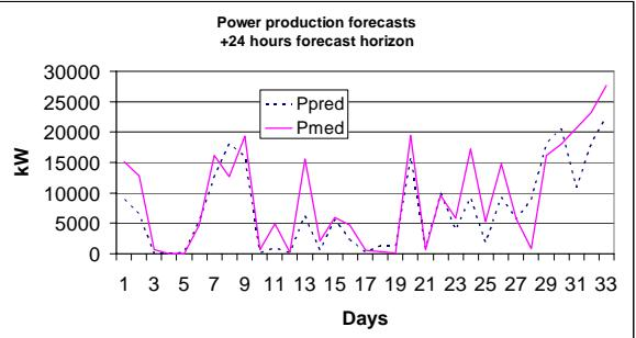
Figure 19. Power production forecasts vs measurements during the validation period. +24 hours forecast horizon.
