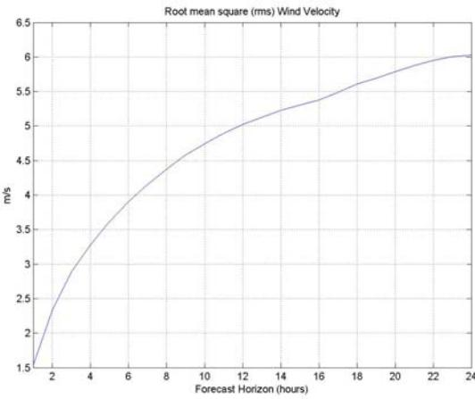
Figure 20: Root mean square error between the AR model and wind speed measurements, forecast horizons between 1 and 24 hours.
