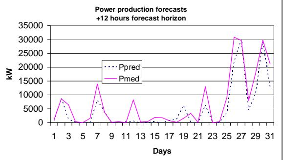
Figure 18. Power production forecasts vs measurements during the validation period. +12 hours forecast horizon. Pmed is measured power, Ppred is predicted power.
