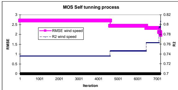
Figure 7. Automatic selection of MM5 variables for the MOS corrections. Evolution of rmse and  $R^2$  of wind speed forecasts for the 12 hours horizon.
