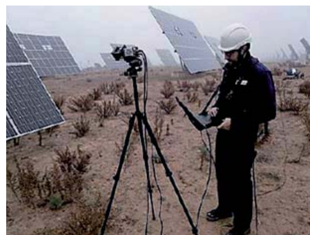
CENER technician taking EL measurement on the field
