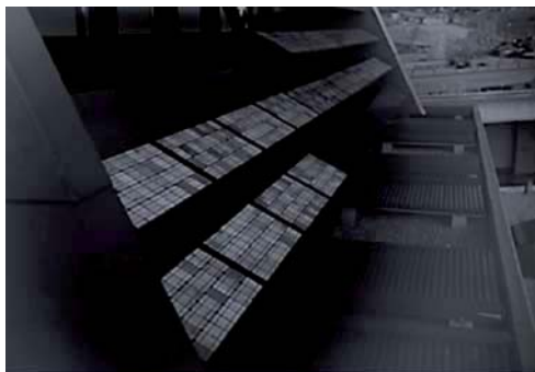
Overlay of visible and EL images of a PV array in a fixed installation integrated in the building facade
