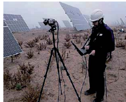
CENER technician taking EL measurements on the field
