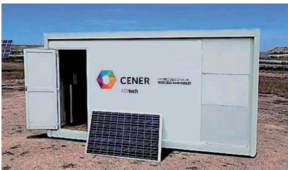
Mobile laboratory to capture EL images of modules at their arrival at the PV plant
