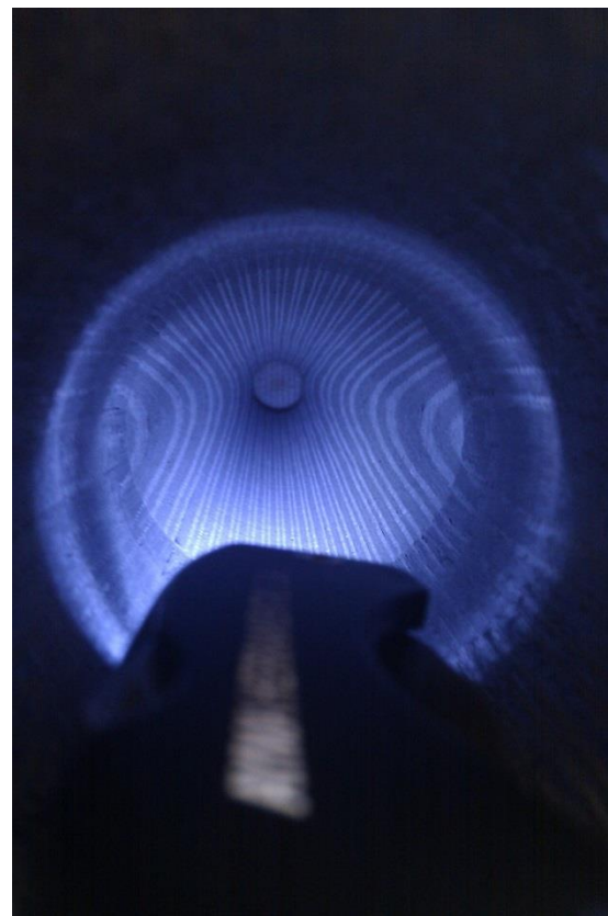
FIGURE 3: Hole dimensional inspection after drilling test on composite material
