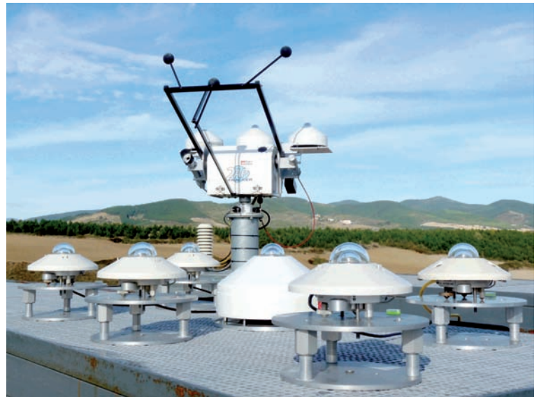
CENER BSRN radiometric station
